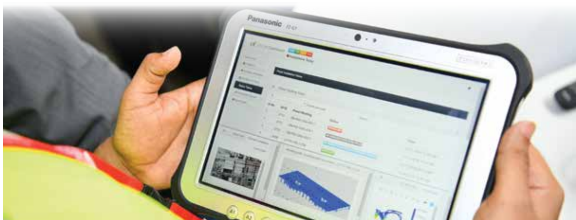
Web-based dashboards display real-time status updates of precast elements, machine productivity and scheduling information.
