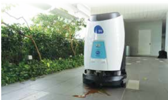
Scrub 50, Singapore's first fully autonomous cleaning solution co-developed by JTC, WIS Holdings and Gaussian Robotics.
