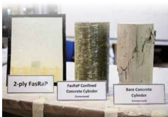
Close up of FasRaP, a concrete pillar wrapped with FasRaP and a cracked bare concrete pillar.
